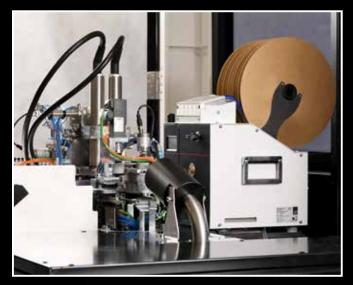
Wire labelling and processing To ensure optimum positioning of the origin/destination on the wires, the Wire Terminal may be fitted with black, white or both marking systems. Multiple insulation stripping and crimping machines may also be integrated using an optional lift.
