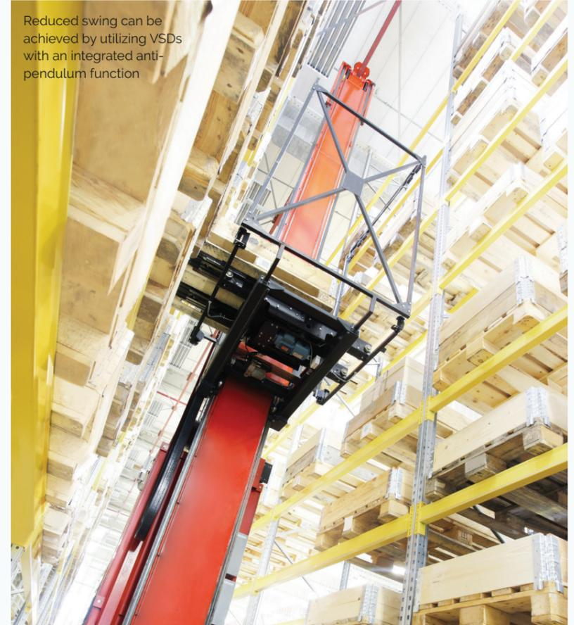
Reduced swing can be achieved by utilizing VSDs with an integrated anti-pendulum function
